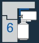
The under-lintle angle (SFW) is being used for installation on the hinge-opposite side if the slide rail needs to be mounted under the door frame (for doors with deep door lintels).
