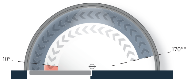
Closing force diagram ECO Newton TS-14, hinge-opposite side
