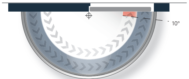
Closing force diagram ECO Newton TS-14 EN, hinge side
