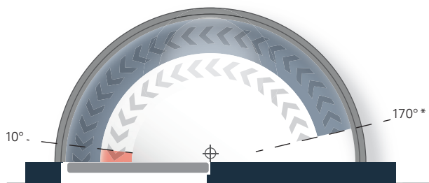
Closing force diagram ECO Newton TS-14 EN, hinge-opposite side
