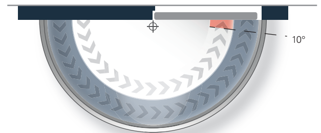
Closing force diagram ECO Newton TS-15 , hinge side
