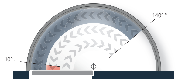
Closing force diagram ECO Newton TS-31, hinge-opposite side
