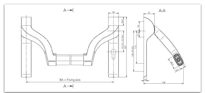
Dimensioning: EPN 900 IV with security long plate counter handle
